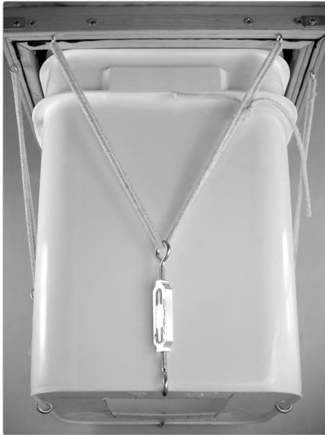
FIGURE 9-12: Detail of the drum's suspension
