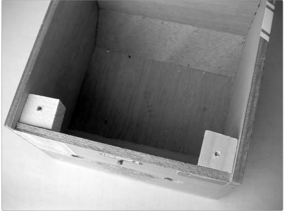
FIGURE 2-4: The blocks installed, with guide holes drilled
