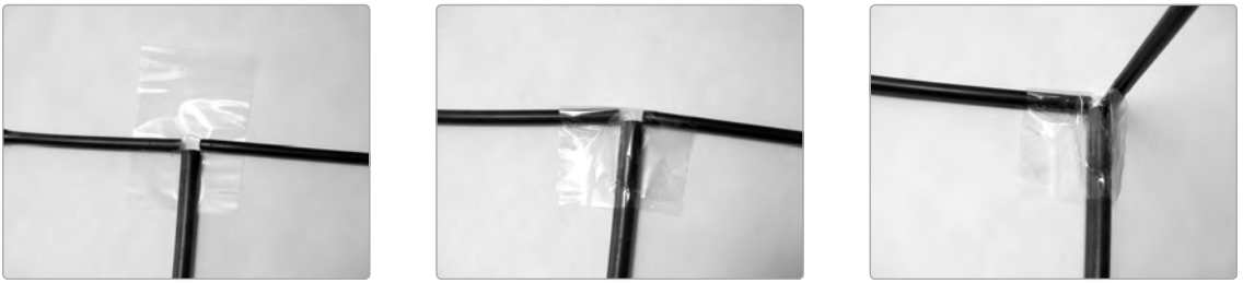
FIGURE 23-20: Secure the cross bars with packing tape and bend them in place.
