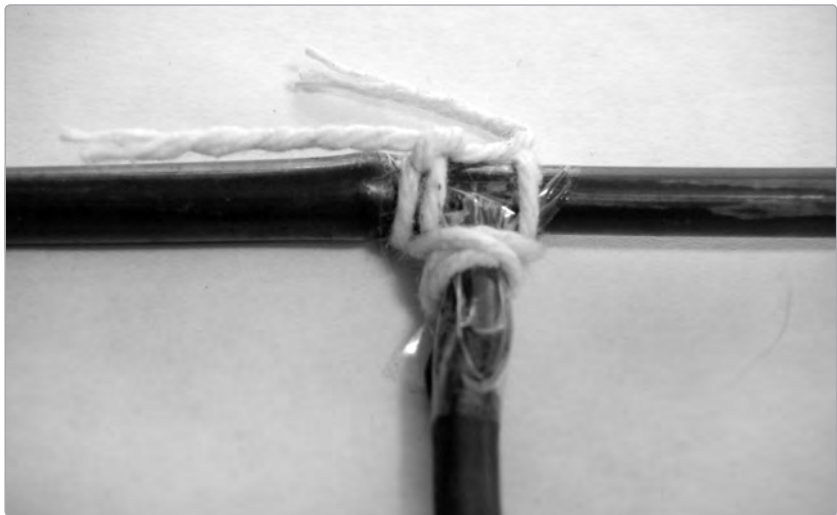
FIGURE 23-18: Wrap the cross braces' joints with string.
