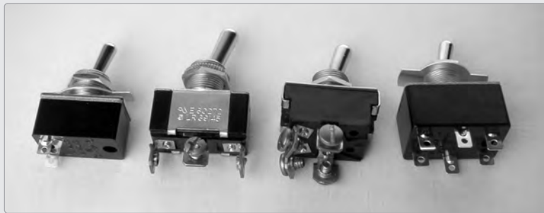
FIGURE 2-8: From left to right, an SPST, SPDT, DPST, and DPDT switch; on the second and fourth switches the common terminals—those shared by the circuits hooked to each pole—are in the middle
