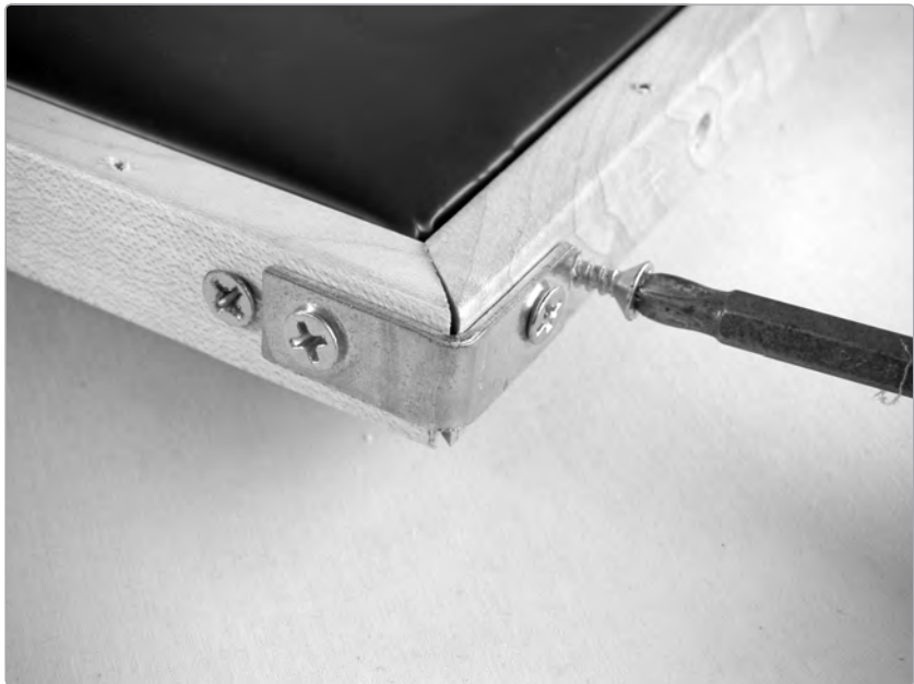
FIGURE 9-8: Securing the frames at the corner
