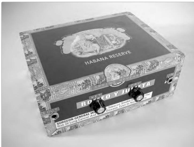
FIGURE 14-1: The finished Spring Reverb
