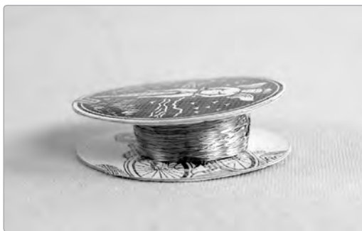
FIGURE 13-15: A freshly wound pickup
