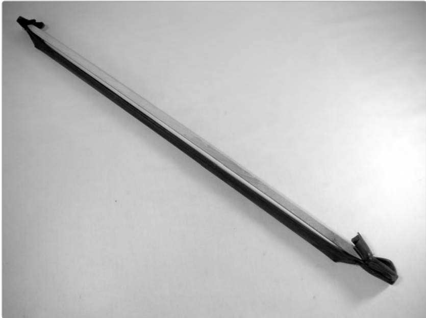
FIGURE 13-23: A homemade bike inner tube bow
