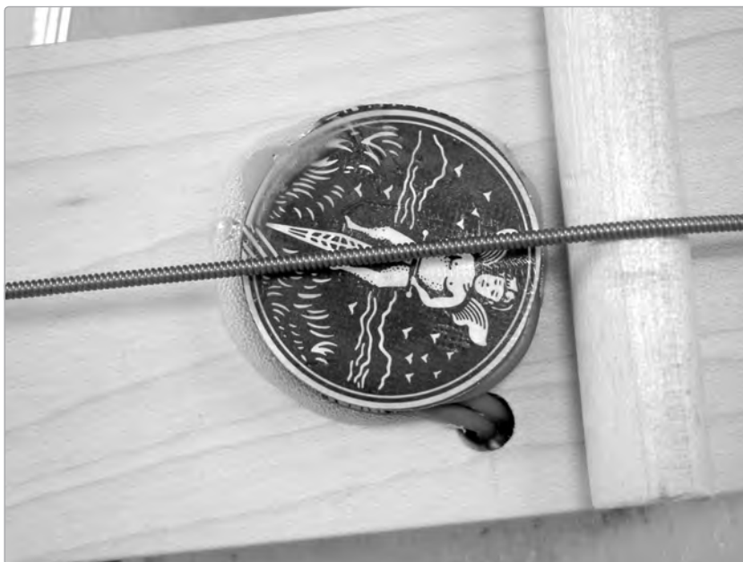
FIGURE 13-19: Detail of an installed pickup; the diddley bow's head is to the left and its butt to the right
