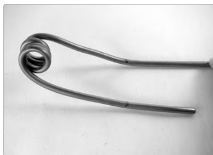
FIGURE 21-8: Bending the tailpipes (left) and a finished boiler coil (right); the tailpipes are bent around 20 degrees (although close is good enough)
