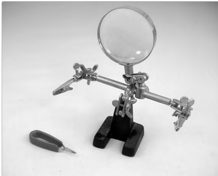
FIGURE A-14: A heat sink (left) and "helping hands" (right)
