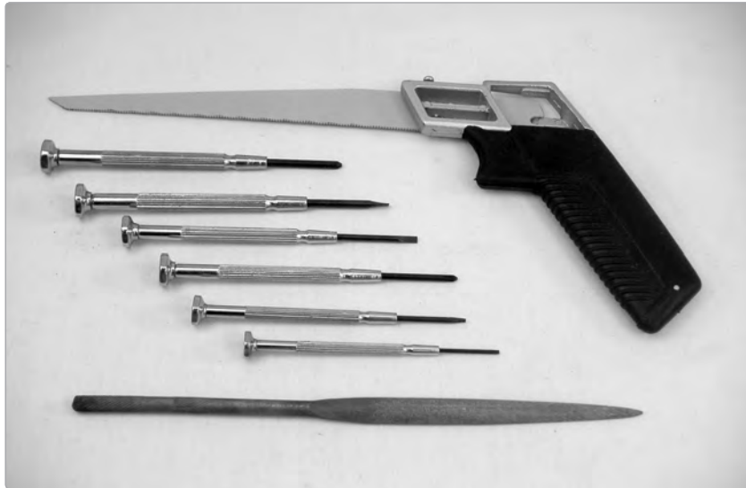
FIGURE A-15: Jeweler's screwdrivers (center), a tapered half-round file (bottom), and a hacksaw (top)
