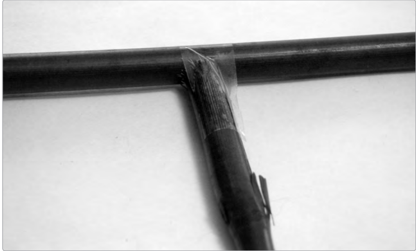
FIGURE 23-17: Secure the cross braces with tape.
