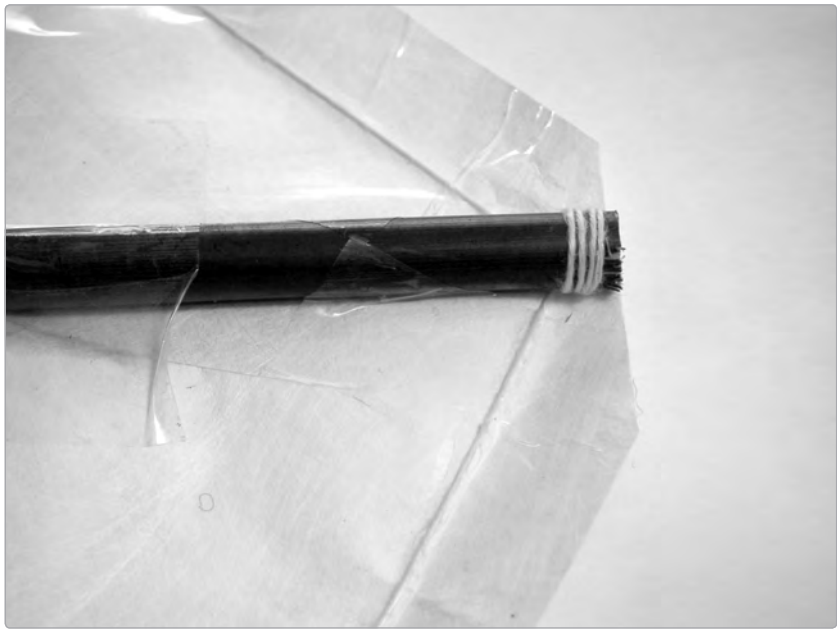
FIGURE 23-11: Detail of a snipped-off diamond vertex
