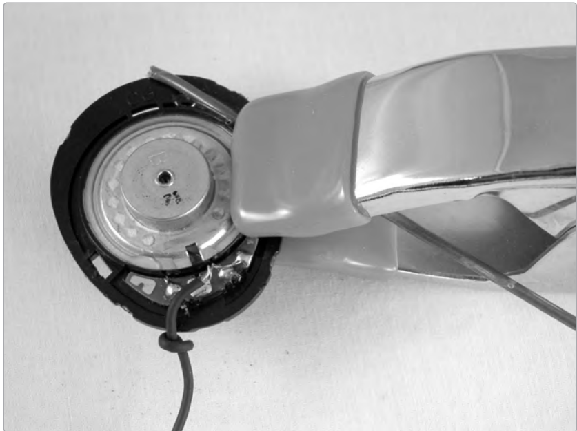
FIGURE 11-13: The pickup, glued and clamped
