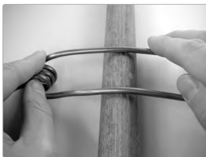
FIGURE 21-8: Bending the tailpipes (left) and a finished boiler coil (right); the tailpipes are bent around 20 degrees (although close is good enough)
