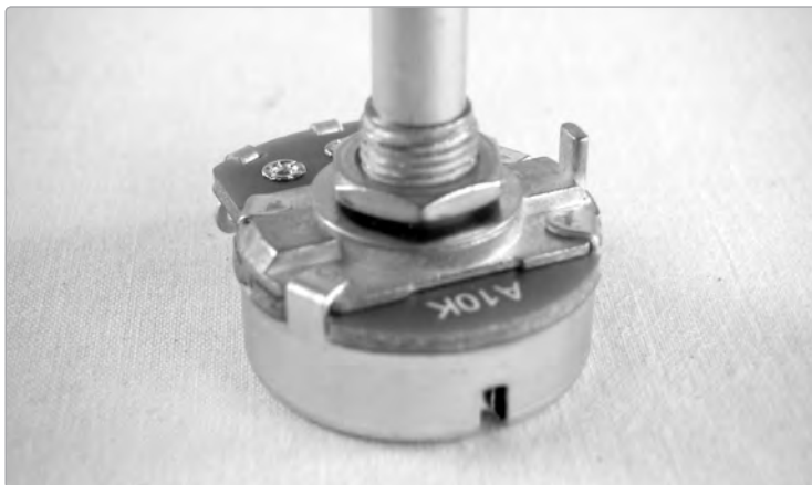
FIGURE 17-12: A close-up of a potentiometer's anchor
