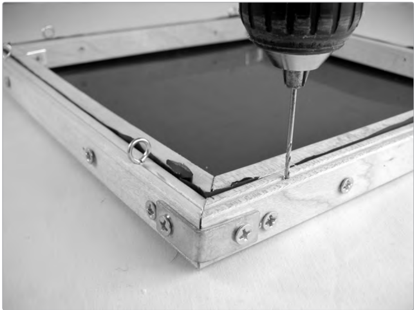
FIGURE 9-10: Drilling a guide hole for a screw eye
