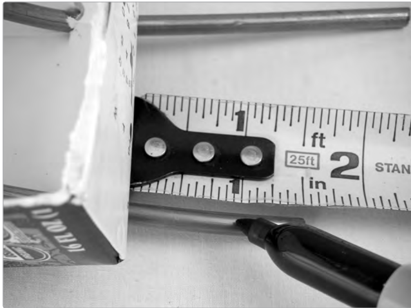
FIGURE 21-9: Marking the tailpipes for trimming
