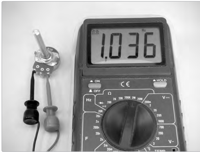
FIGURE A-23: Identifying a potentiometer
