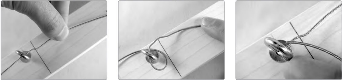
FIGURE 13-11: The three steps to properly stringing any steel-stringed instrument: (1) Give 1" of slack, (2) Pass the free end under, and (3) Kink it up
