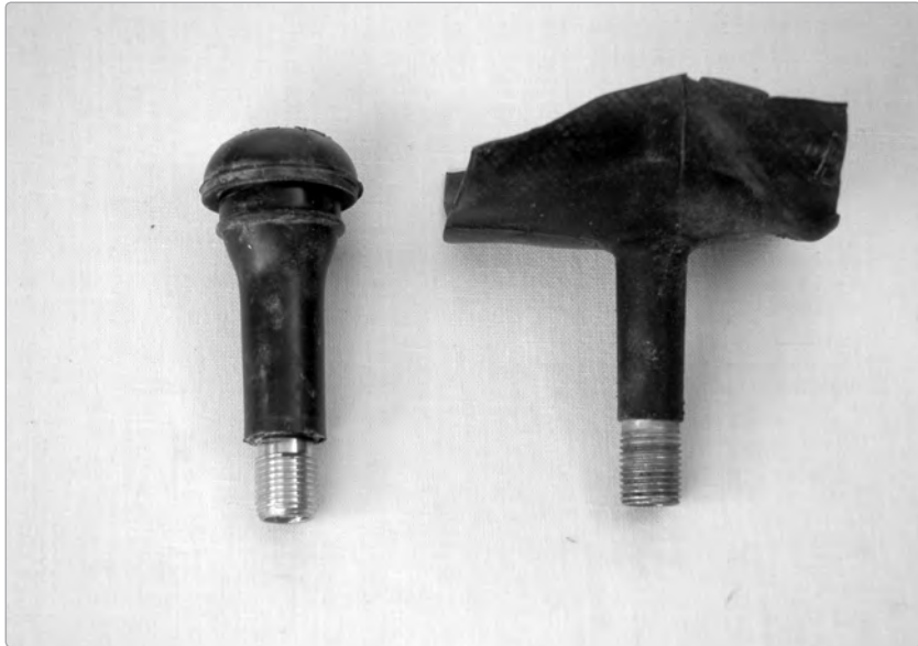
FIGURE 20-3: A car tire stem (left) and bike tire stem (right); most of the inner tube has been cut away from the bike stem—you'll need to cut it all away to build your launch plug
