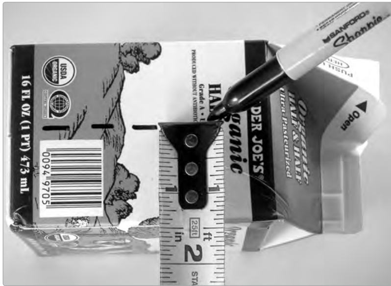
FIGURE 21-3: Marking the carton for cutting; the “front” of the carton is at the top of the photo, the “back” is at the bottom, and the dashed line continues around the bottom of the carton (i.e., the left end) and along the other side
