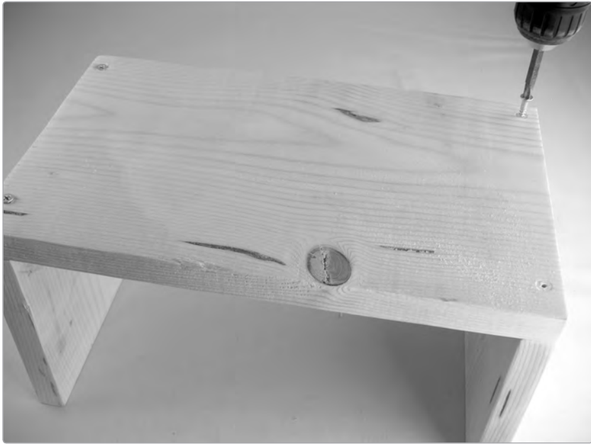
FIGURE 1-5: Installing the bottom; note the pre-drilled guide hole in the front right corner
