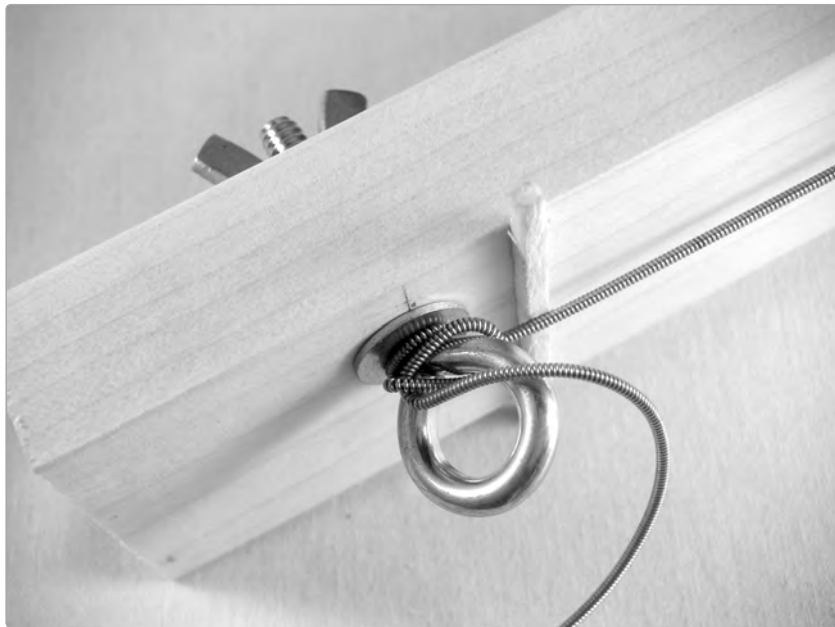
FIGURE 13-12: A properly wound string with floating matchstick nut
