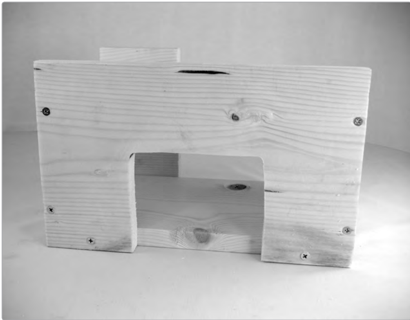
FIGURE 1-6: The back installed (the anchored side of the barn door, attached to the left end piece, is also visible)
