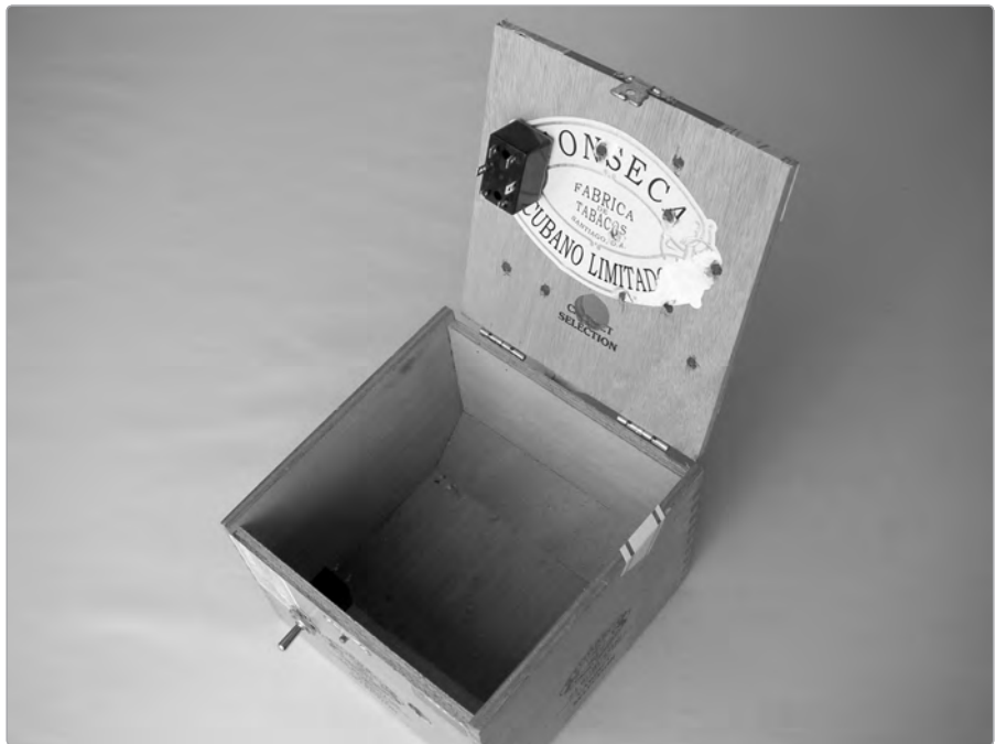
FIGURE 2-3: The drilled box with two switches in place
