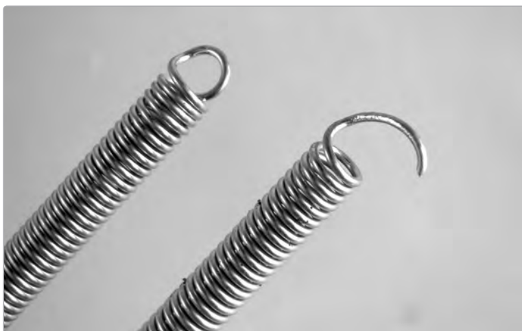
FIGURE 10-5: The end of the spring before (left) and after (right) being opened into a hook
