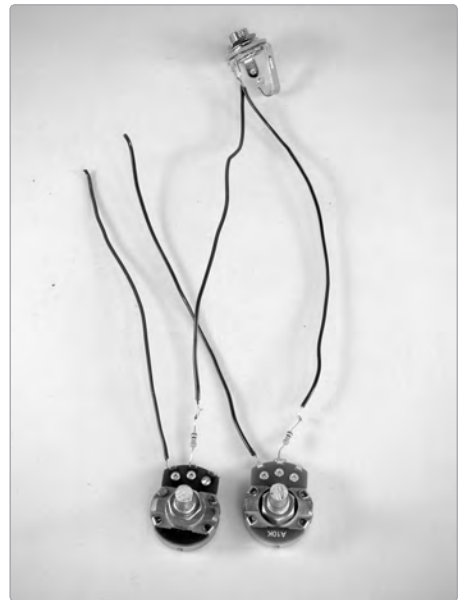
FIGURE 14-4: The reverb's two-channel mixer
