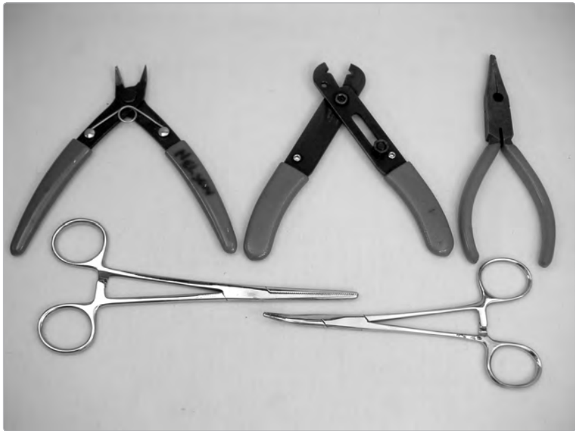
FIGURE A-12: Clockwise from top left: diagonal cutters, wire strippers, needle-nose pliers, and two types of clamps
