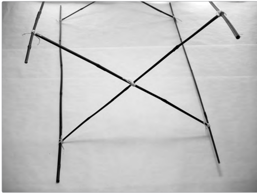
FIGURE 23-19: The top cross braces secured with string
