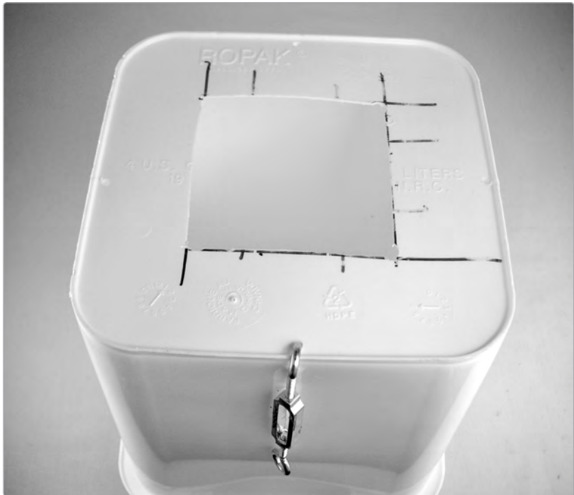
FIGURE 9-11: The bottom of the bucket with one turnbuckle installed
