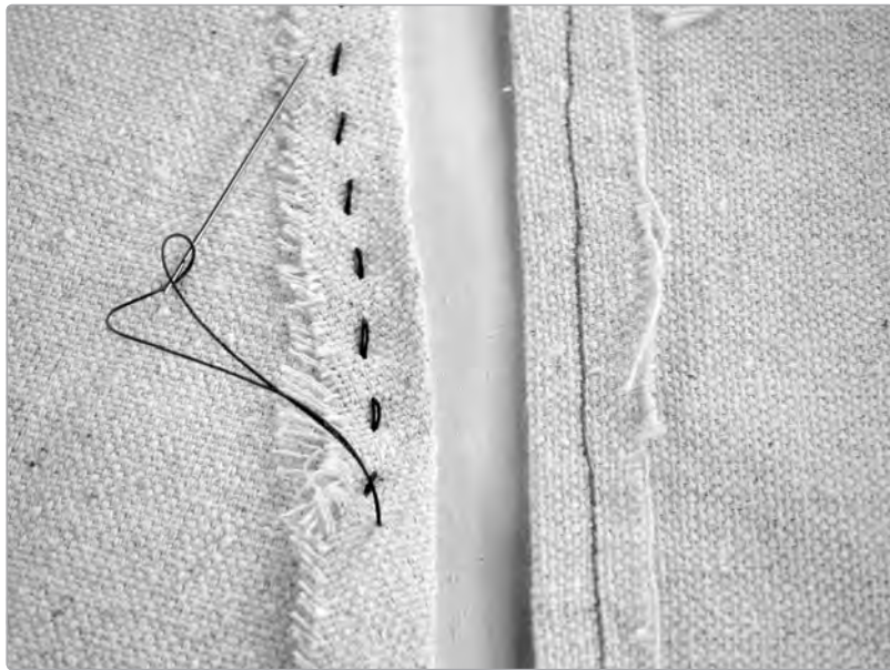
FIGURE 4-9: On the left is a hand-sewn hem using a running stitch; on the right is a hem that's been sewn using a sewing machine.
