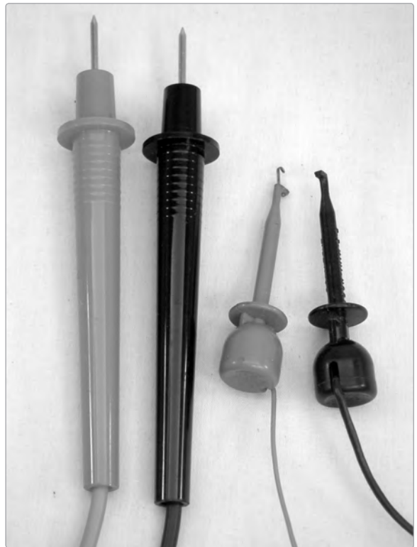
FIGURE A-17: A set of probes (left) and mini-clip leads (right); the latter are retractable hook leads, also called mini-clip jumpers, and are easy to clip to the leg of a single PCB-mounted component without creating a short circuit
