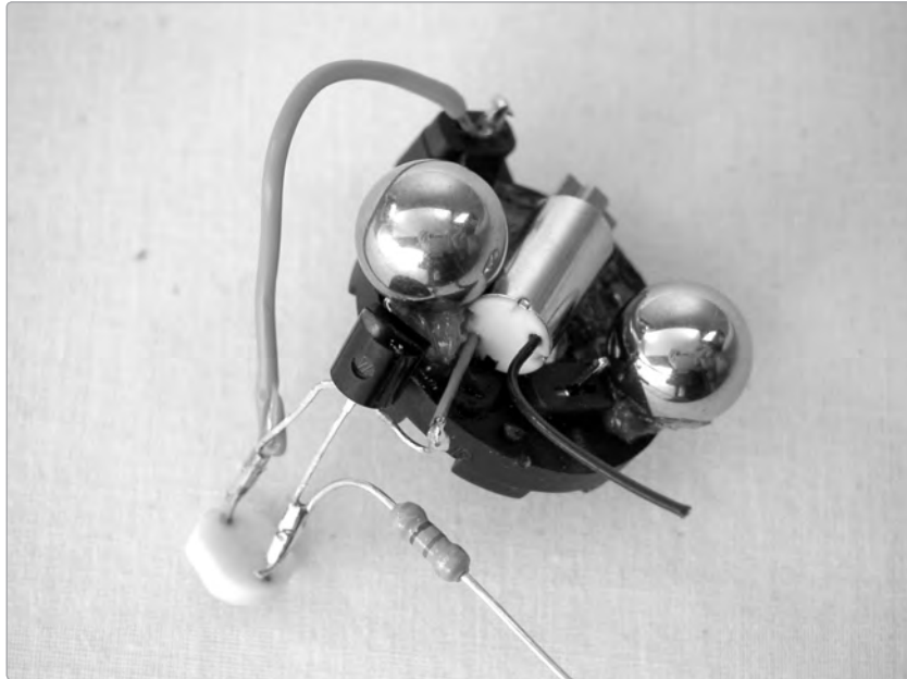
FIGURE 22-9: The transistor soldered to the motor
