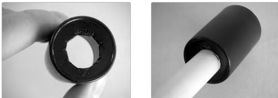
FIGURE 24-5: The prepared canister (left)—notice how ragged the hole is—and the barrel and chamber (right)
