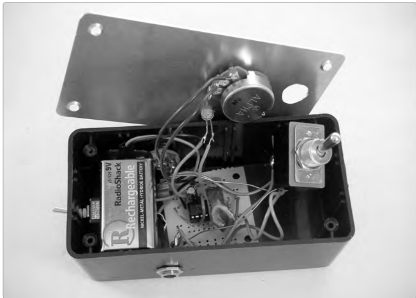
FIGURE 15-12: The packaged effect, innards exposed
