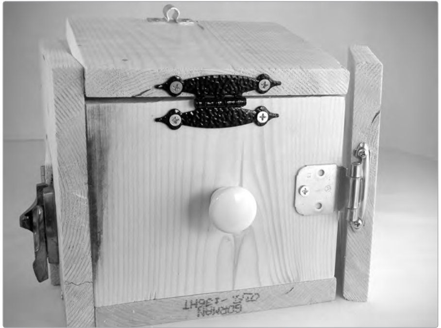
FIGURE 1-7: Hinge orientation for lid (top) and barn door (right)
