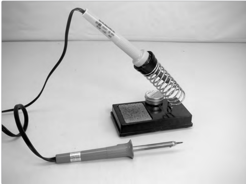
FIGURE A-11: Here are a 15-watt (bottom) and 25-watt soldering iron with stand (top). The damp sponge in the stand is used for cleaning the tip, although many tinkerers prefer to use a copper scrubbing pad or old bolt instead.
