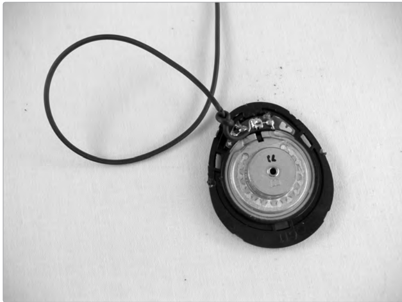
FIGURE 11-11: A gutted headphone earpiece
