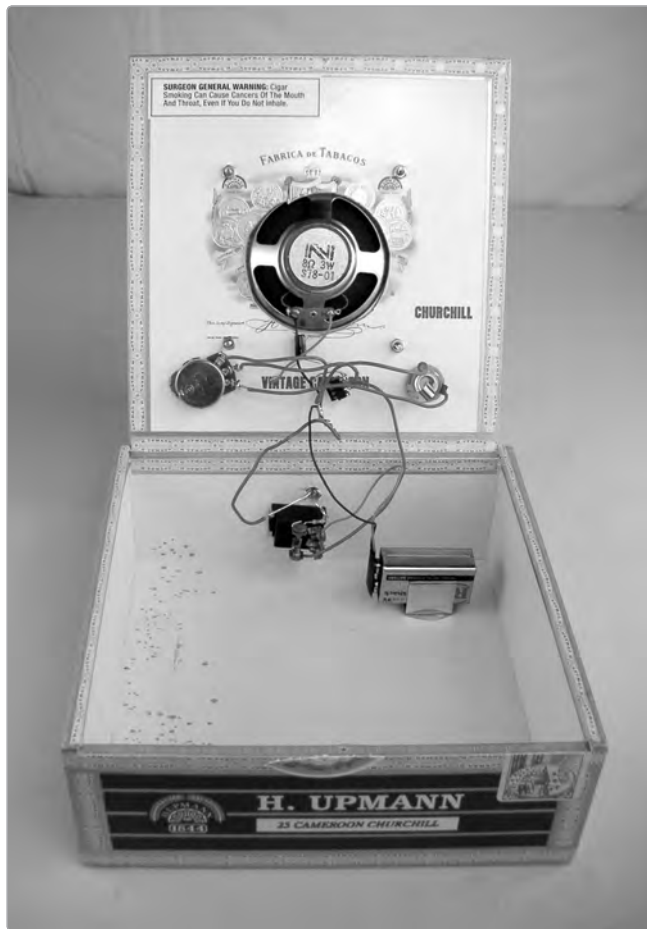
FIGURE 12-12: The finished amp guts installed
