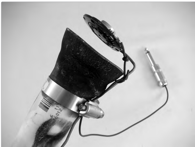
FIGURE 11-17: A good position for our homemade limited-range mic pickup
