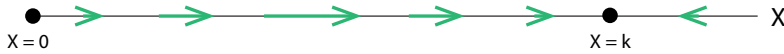
Figure 1.36: The vector field for the logistic equation, X' = rX(1 - \frac{X}{k}) , with r = 0.2 and k = 100 .
